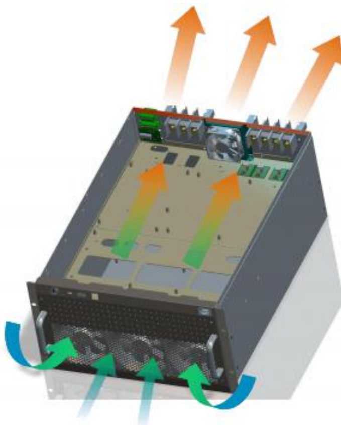
Figure 4-1 Heat dissipation of the rear terminal
